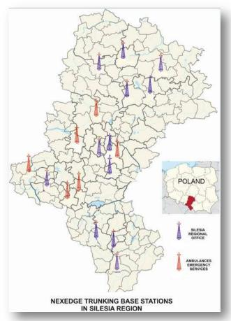
The NEXEDGE trunked system we designed and implemented employs 17 sites located on mast or high buildings and one site within a highway tunnel with leaky feeders. These are all connected via IP by fiber optic. We also provided an additional mobile site for rapid deployment by the Regional Crisis Management Centre in emergency situations which is connected to the system by IP using LTE/CDMA450".
